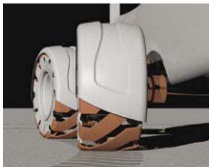
Four-wheel steering will ensure turning impact is limited to two footprints
