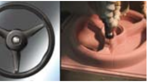
ABOVE: MDI concept sketch and CNC machining operation for new steering wheel
